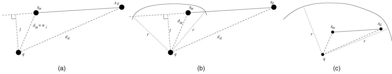
Fig. 11. An example of Case 2 ( $n_i = d_{in}$ ) Line-Segment Uncertainty. (b) Intersection by  $C_q(r)$  with radius  $r$ , centered at  $q$ , such that  $d_{in} \leq r \leq d_{il}$ . (c) Intersection by  $C_q(r)$  with radius  $r$ , centered at  $q$ , such that  $r > d_{il}$ .
